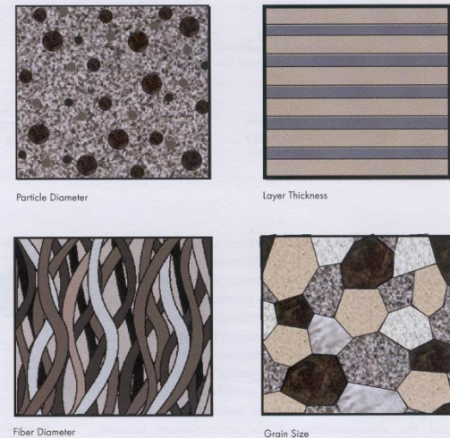
Figure 1. Nanostructured Materials are Characterized by the Inclusion of One or More Types of Features with Dimension Below 100 Nanometers
