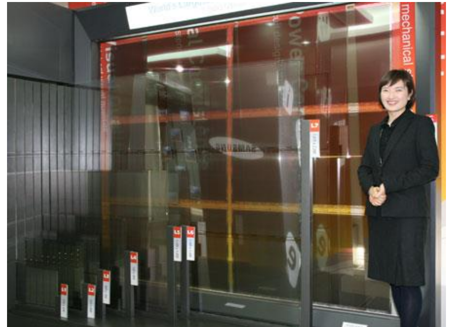
Generation 8 glass panel patterned with six backplanes for 52" Samsung televisions. Previous generation glass panels are seen to lower left.
