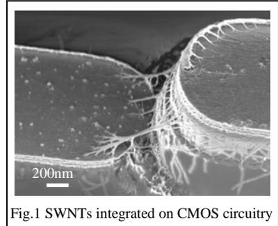
Fig.1 SWNTs integrated on CMOS circuitry
